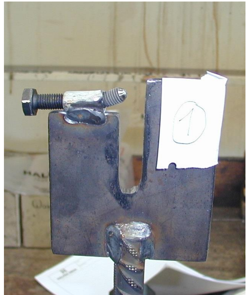
Testing Pointed (Fixed) Bolts – 50Nm Torque – Average Failure Load 8.8 kN
